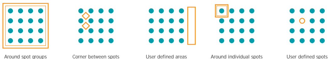
Fig 83. Some of the background region options available to the user in the ArrayVision™ Image Analysis Software. The green represents the spots enclosed by the grid while the blue encloses the background region. Image analysis quality metrics calculated by analysis software are increasingly used to highlight data that may be unreliable and should be omitted from further analysis. Typical causes of suspect data include dust speckles over spots, poor spot morphology, very low or very high signal.
